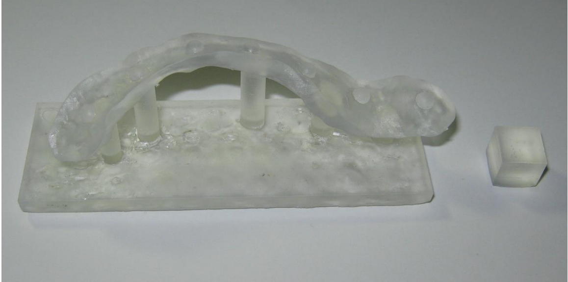
Figure 27 - Proof of Process Bending Template and Isotropic Cube.
