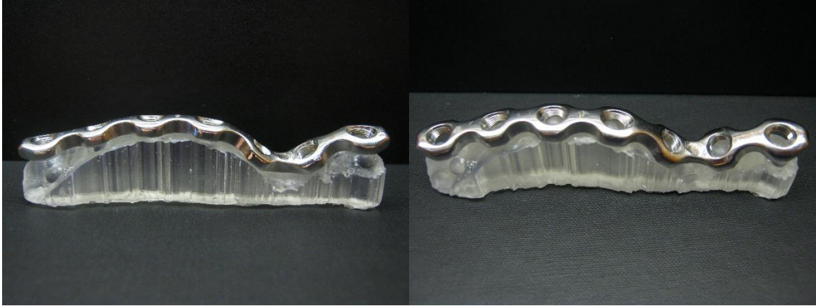
Figure 26 - A Reconstruction Plate Bent to an Initial Bending Template.
